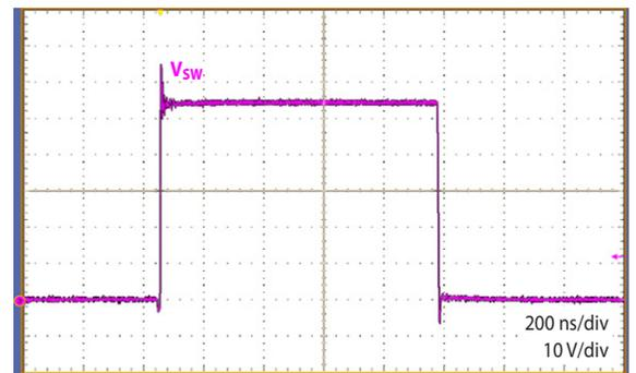
Figure 5. Switch-node voltage  $v_{sw}$  waveform at 12.5 A output current
